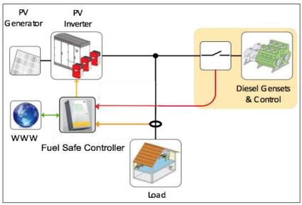
Figure 15: Intelligent and fast interface between load, generator and PV inverter - Fuel Save Controller (SMA Solar Technology)
